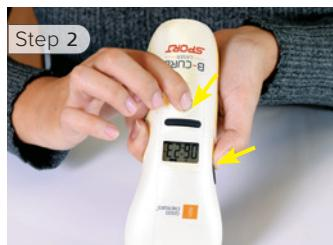
Continue pressing and simultaneously press using an additional finger on the pressure switch area
